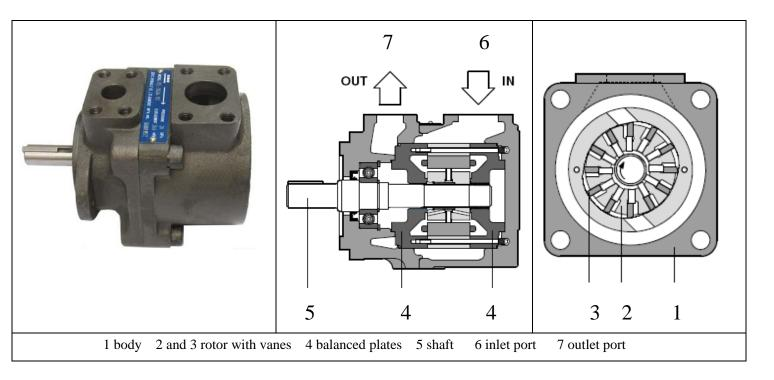
PFE are fixed displacement-twelve-vane pump, 2 and 3 cartridge design with integral hydraulic balancing 4 for high pressure operation and long service life with low noise level.
